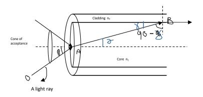
Consider a light ray falling in to the optical fibre at an angle of incidence  $\theta_0$  equal to acceptance angle. Let  $n_0$  be the refractive index of the surrounding medium .
