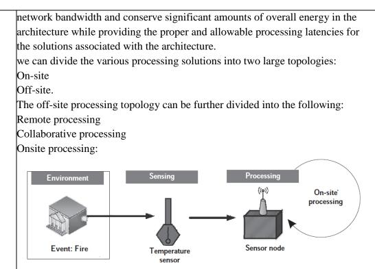
As evident from the name, the on-site processing topology signifies that the data is processed at the source itself. This is crucial in applications that have a very low tolerance for latencies. These latencies may result from the processing hardware or the network (during transmission of the data for processing away from the processor).
