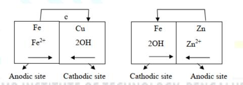
*Case 1*: The standard electrode potential of Fe is – 0.44 V which is less than that of Cu whose standard electrode potential is 0.34 V. Hence in this case iron acts as anode and undergoes corrosion whereas copper acts as cathode and remains unaffected.
