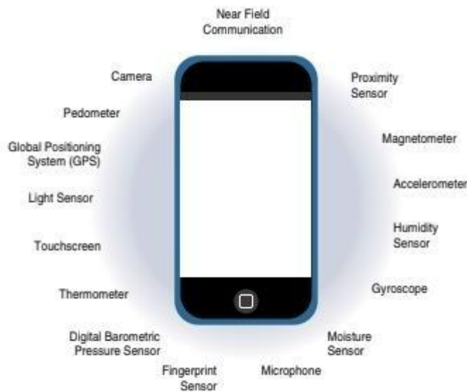
Figure 3-2 Sensors in a Smart Phone
