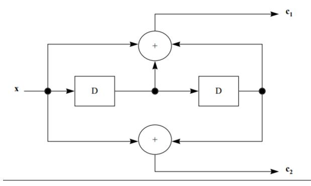
The conventional convolutional encoder is represented by the generator sequences g1 = [111] and g2 = [101] and can be equivalently represented in a more compact form as G=[g1, g2]. The RSC encoder of this conventional convolutional encoder is represented as G=[1, g2 / g1] where the first output (represented by g1) is fed back to the input. In the above representation, 1 denotes the systematic output, g2 denotes the feedforward output, and g1 is the feedback to the input of the RSC encoder.
