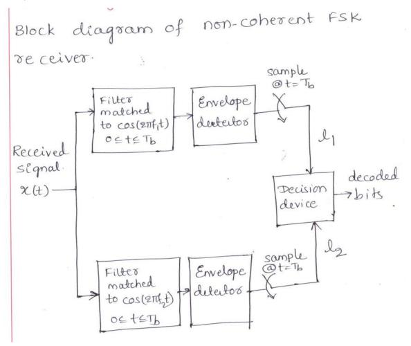
The non-coherent receiver consists of
