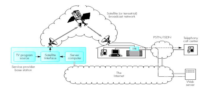
The STB associated requires a high speed modem to provide the connections to the PSTN and the Internet.
