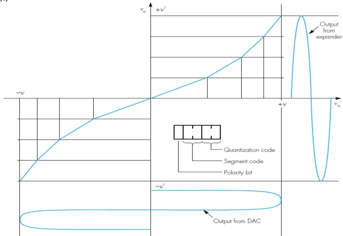
Note that in the G.711 standard a 3-bit segment code and 4-bit quantization code are used.
