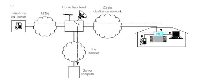
The set-top box (STB) provides both a low bit rate connection to the PSTN and a high bit rate connection to the internet
