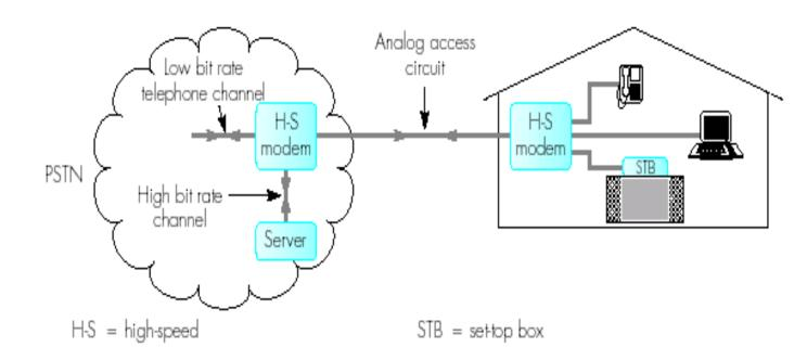
Today with *high bit-rate channels* in addition to the voice using the same access networks high resolution audio and video can be downloaded from a range of entertainment related servers.
