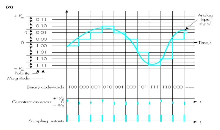
Three bits are used to represent each sample (1 bit for the sign and two bits to represent the magnitude)
