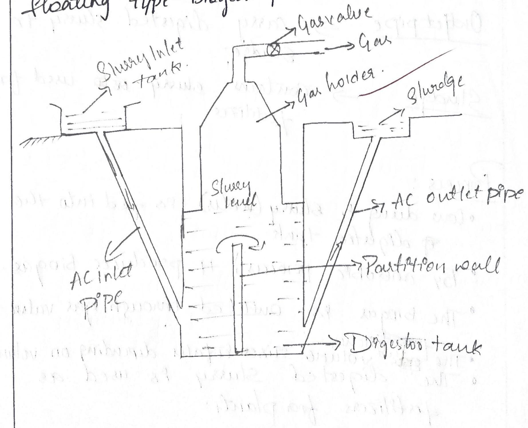
Slurry inlet tank → collects Cow dung & water (slurry)
