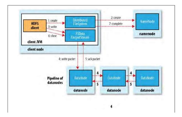
DFSOutputStream also maintains an internal queue of packets that are waiting to be acknowledged by datanodes, called the ack queue. A packet is removed from the ackqueue only when it has been acknowledged by all the datanodes in the pipeline (step 5).
