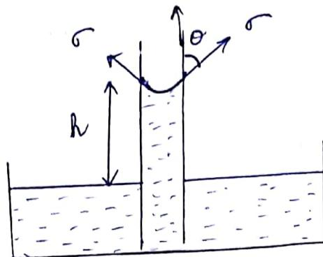
Consider a glass tube of small diameter 'd' open at both ends and inserted in a liquid.
