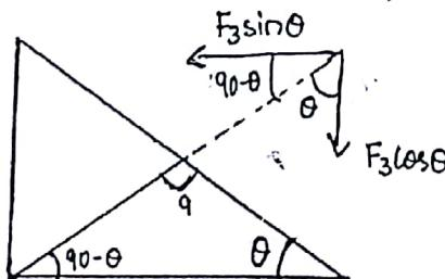
$$F_4 = mg = \text{volume} \times g = \frac{1}{2} \times dx \times dy \times l \times g$$
