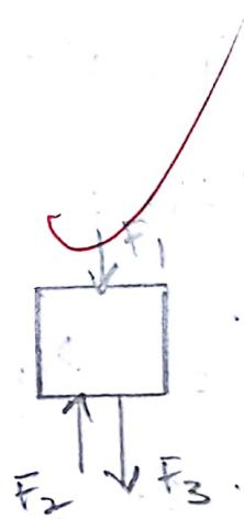
From the figure above, by applying equilibrium conditions, hydrostatic law can be proved as  $P = \rho g \cdot h$ .
