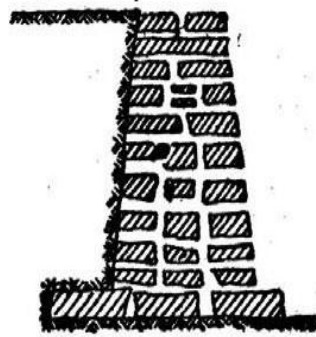
Dry Rubble masonry
