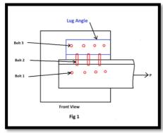
A single ISA  $75 \times 50 \times 8$  is connected (longer leg) with gusset plate using use 4 bolts of 20 mm diameter in one line at pitch of 50 mm and edge distance of 30 mm. What is the Design tensile strength due to block shear failure? (Assume gauge distance = 35 mm)
