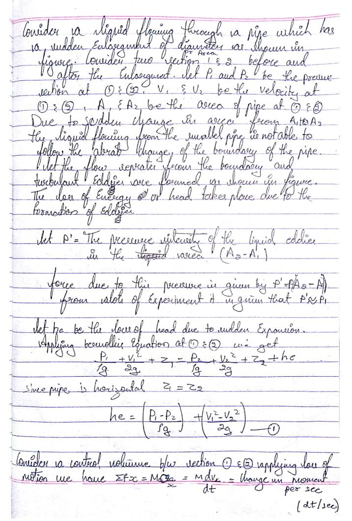
E Fx = Change in nomentum EFX = P. A. + P' (A2-A1) = P3 A2  $P' \approx P_0$ = P, N, + P, A = P, A, + Pa A = = Aa(P, +Pa) >Fx = A(P1-P2) PARVa2-PAIVI2 Equating 3 & D (P, -Pa) Aa = /Aa Va2 - JA, V,2  $Q = A_1 V_1 = A_2 V_2 \Rightarrow A_1 = A_2 V$ (P,-P2) P2 = PA= 13 2- PA= 14 12 V, P1-P2) = V22 - V2V1 Sub (5) in (1) = 21/2-21/21/14/2-192
