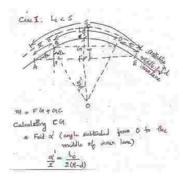
A state highway passing through a rolling terrain has a horizontal curve of radius equal to the ruling minimum radius. Design all the geometric features of this horizontal curve, assuming suitable data. Specify the minimum set-back distance from the center line of the two lane highway on the inner side of the curve up to which the buildings should not be constructed so that ISD is available throughout the circular curve. Assume the length of the circular curve is greater than the sight distance.
