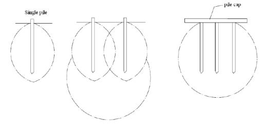
Generally center to center spacing between piles in a group is kept between 2.5 d and 3.5d where d is the diameter of the pile.
