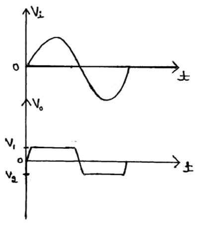
1b. Analyse the circuit and draw the pattern of the output  $(V_{\text{o}})$  of the circuit shown in figure .
