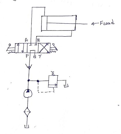
the cylinder is highsaulically locked and the pump is unloaded back to the tank.
