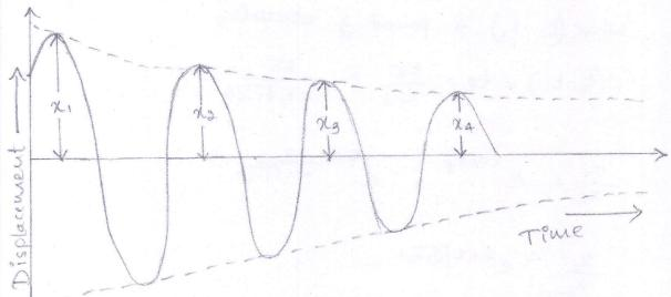
Displacement of an underdamped system in given as
