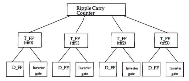
In a top-down design methodology, the functionality of the ripple carry counter is specified, which is the top-level block. Then, the counter with T \_FFs is implemented. The T \_FFs are built using D \_FF and an additional inverter gate. Thus, the bigger blocks are broken into smaller building sub-blocks until further breakup of the blocks is not possible.
