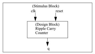
The second style of applying stimulus is to instantiate both the stimulus and design blocks in a top-level dummy module. The stimulus block interacts with the design block only through the interface.
