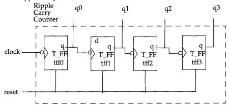
Each of the T-FFs can be made up from negative edge-triggered D-flipflops (D-FF) and inverters.
