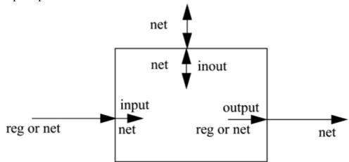
One can visualize a port as consisting of two units, one unit that is internal to the module and another that is external to the module. The internal and external units are connected. There are rules governing port connections when modules are instantiated within other modules. The Verilog simulator complains if any port connection rules are violated.
