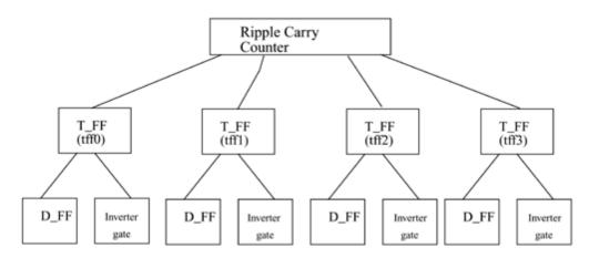
There are two basic types of digital design methodologies: a top-down design methodology and a bottom-up design methodology. In a top-down design methodology, we define the top-level block and identify the sub-blocks necessary to build the top-level block. We further subdivide the sub-blocks until we come to leaf cells, which are the cells that cannot further be divided. Above figureshows the top-down design process.
