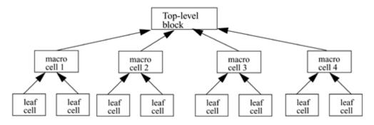
In a bottom-up design methodology, we first identify the building blocks that are available to us. We build bigger cells, using these building blocks. These cells are then used for higher-level blocks until we build the top-level block in the design.
