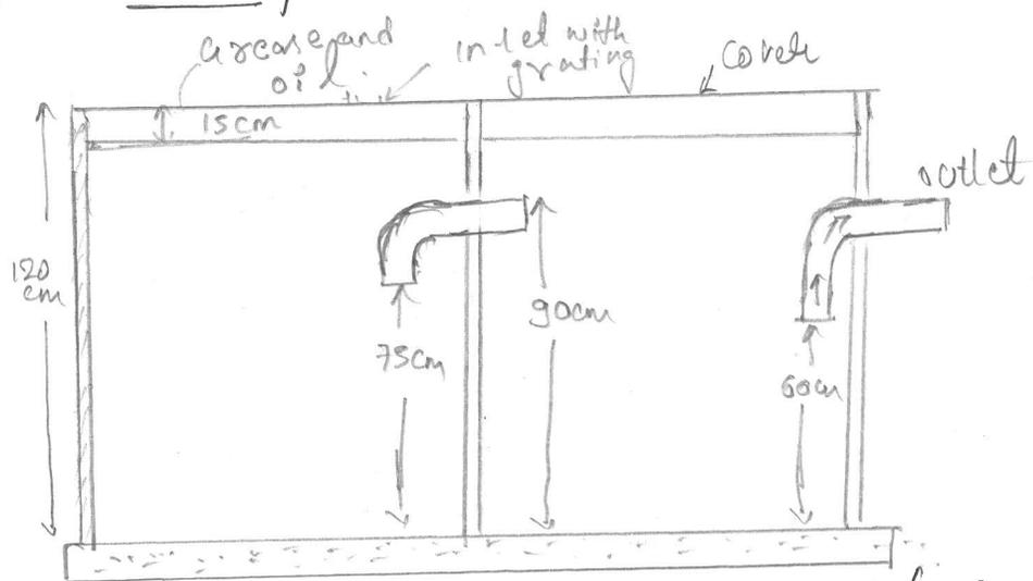
The w/w from kitchen or hotel, restaurants, industries - consists of oil, grease & fat. If these are not removed they will stick to the interior surface of the sewer and sewer gets clogged. Some from garages particularly from the floor drains & wash racks contain oils, mud & sand.
