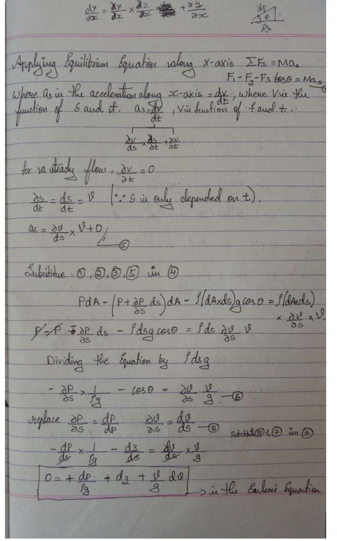
By integrating the Equation.  $\int \frac{dP}{fg} + \int \frac{dz}{g} + \int \frac{v}{g} dv = 0$ P + Z + V2 - Constant P in the perelever head in noters. in the daltown or potential head. 12 in nelocity or finetic head in moters. Energy head = Energy weight and continues, hum of perecure head, KGH and Poly is a louetout along is a stream line. fg + 3 + V2 - benefaut
