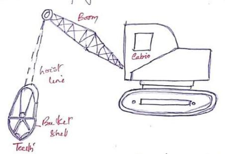
Since the bucket is like a class fish and has hinged double shell, it is named as classished.
