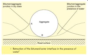
**Detachment:** Detachment occurs when a thin film of water or dust separates the bitumen and aggregate with no obvious break in the surface of the bitumen film being apparent. Although the bitumen film completely encapsulates the aggregate particle, no adhesive bond exists and the bitumen can easily be peeled from the aggregate surface.
