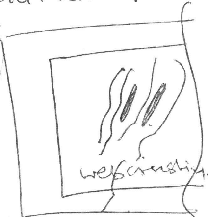
web crushing. web compression failure.
