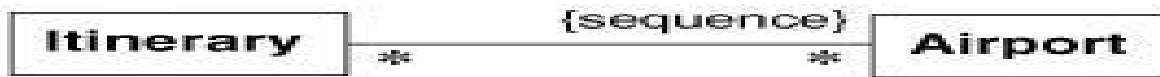
Figure 3.16 An example of a sequence. An itinerary may visit multiple airports, so you should use {sequence} and not {ordered}.
