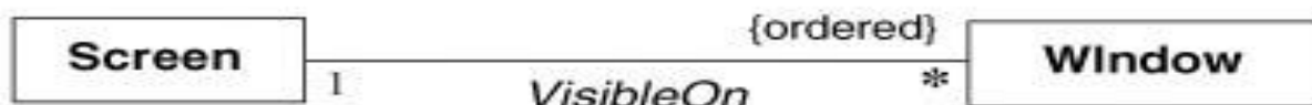
Figure 3.15 Ordering the objects for an association end. Ordering sometimes occurs for "many" multiplicity.
