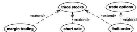
Figure 8.2 Use case extension. The extend relationship is like an include relationship looked at from the opposite direction. The extension adds itself to the base.
