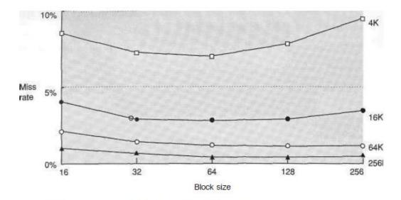
Miss rate versus block size for five different-sized caches. Note that miss rate actually goes up if the block size is too large relative to the cache size.
