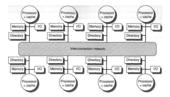
Before we see the protocol state diagrams, it is useful to examine a catalog of the message types that may be sent between the processors and the directories for the purpose of handling misses and maintaining coherence
