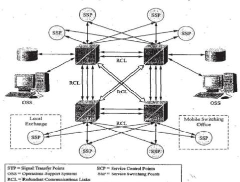
SS7 network. All SS7 data packets travel from one service switching point to another through signal transfer points that serve the network as routers, directing the packets to their proper destination. There are several different types of redundant links between the signal transfer points to provide the SS7 network with a high degree of reliability.
