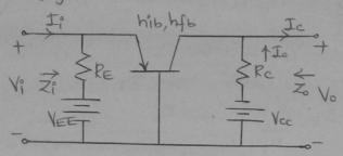
(b) CB configuration using b-parameters:
