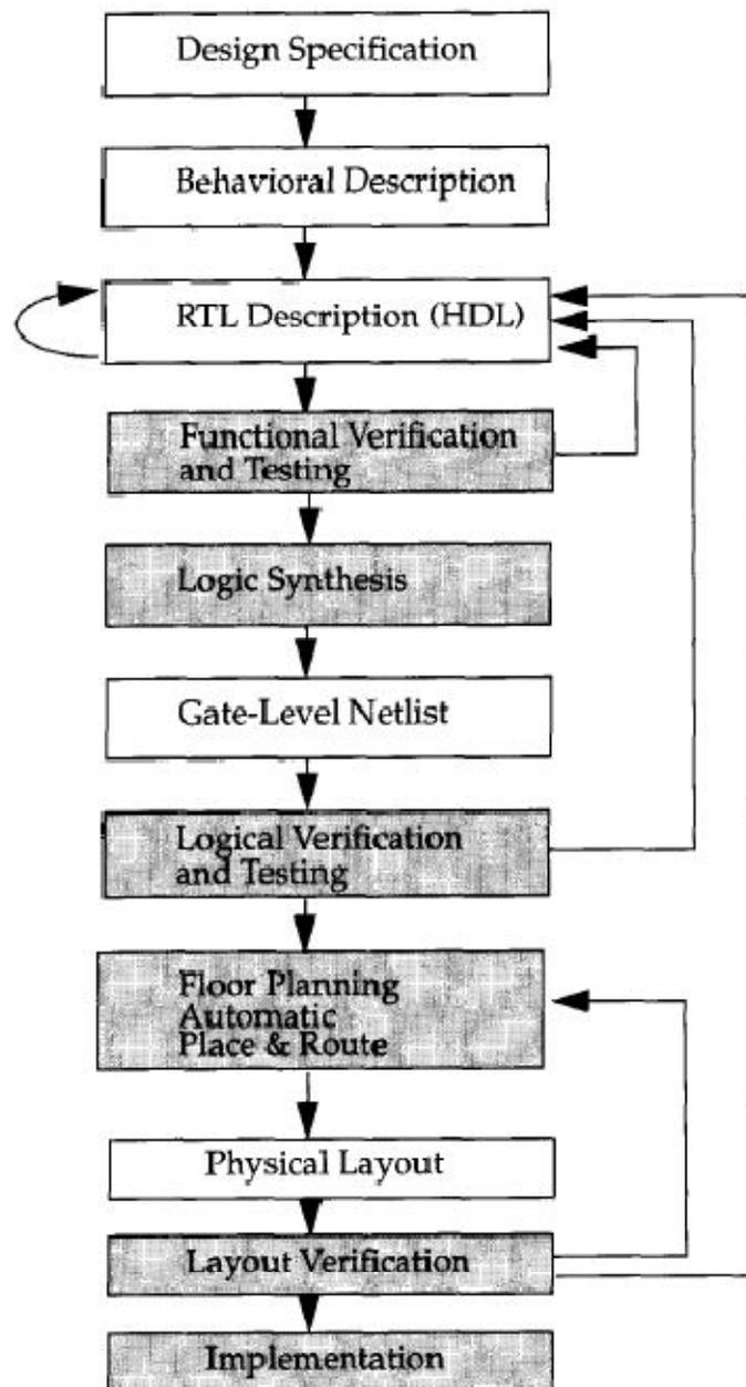
Any design starts by writing the specification first. Specifications describe the functionality, interface and overall architecture of the digital circuit to be designed. Without working on the implementation.
