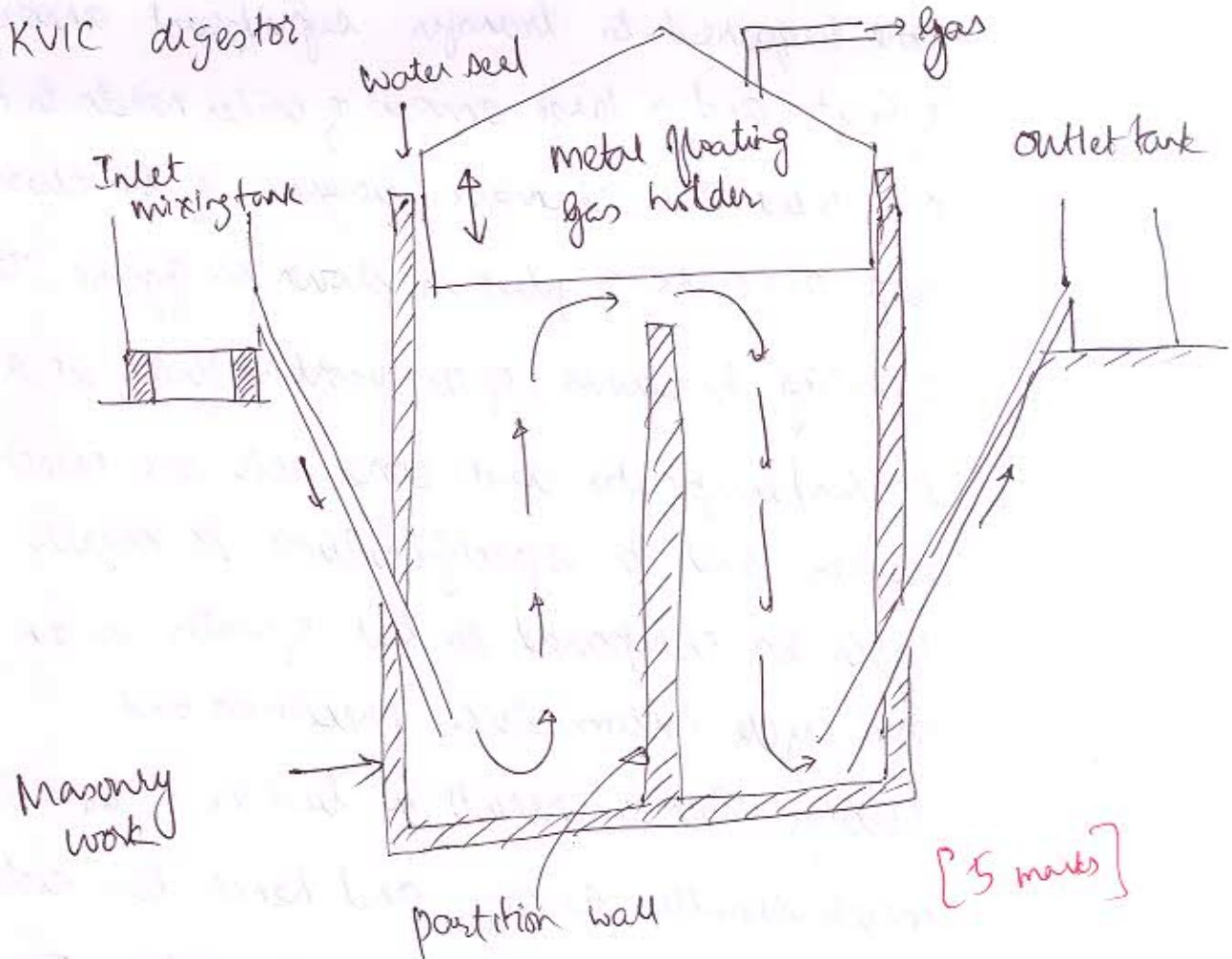
The KVIC model (Khadi and Village Industries Commission) consists of an inverted mild steel drum to work as gas holder. The digester is an underground masonry construction with a partition wall. The bifurcation of a  $\text{pH}$  digestion chamber through a partitioning wall provides optimum conditions for growth of acid formers and methane formers as the pH values for these bacteria are different.
