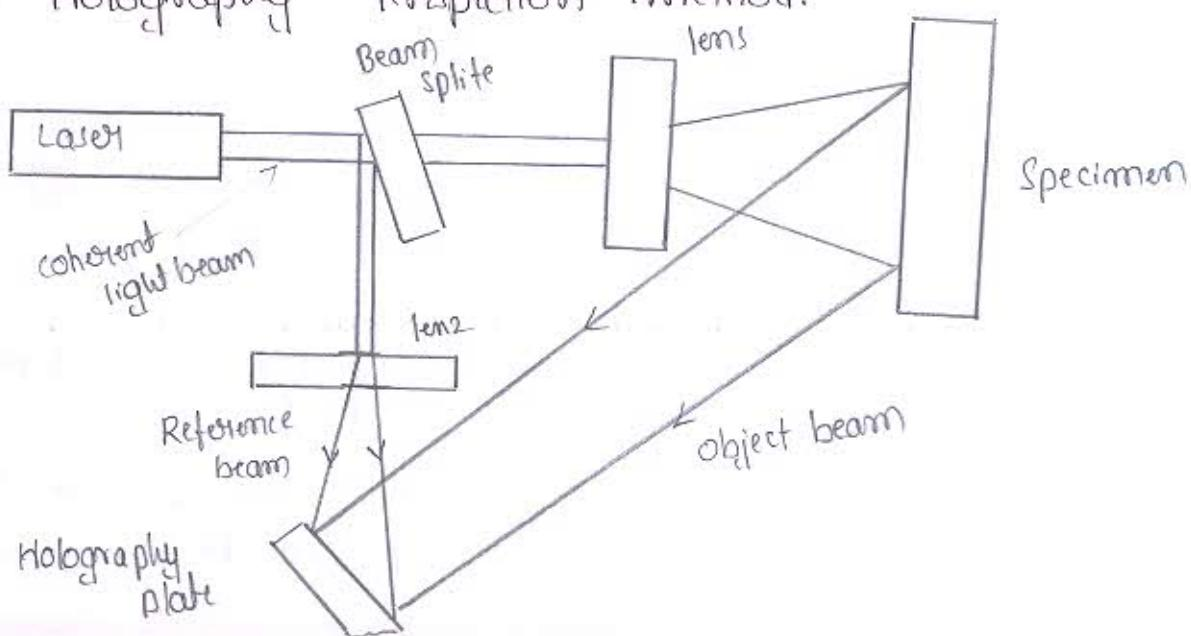
Figure shows the arrangement of holographic interferometry for the inspection of parts having shapes and surface conditions.
