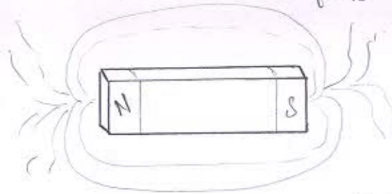
Magnet with flux leakage
