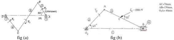
3 Determine torque  $T_2$  to keep the mechanism in equilibrium shown in fig (b).
