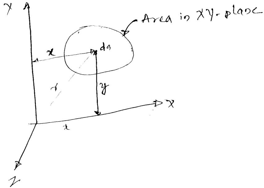
If a plane lamina lies in the XY plane as shown in figure. Then the axis perpendicular to XY plane is Z-axis. The moment of inertia of an area about an axis perpendicular to its plane is known as Polar moment of inertia.
