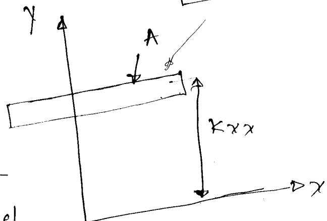
If the area shown in fig is concentrated into a strip of the same area and is placed parallel to x-axis at a distance of  $K_{xx}$  as shown, such that this strip has the same moment of inertia about x-axis as that of area A, then  $K_{xx}$  is known as the radius of gyration about x-axis.
