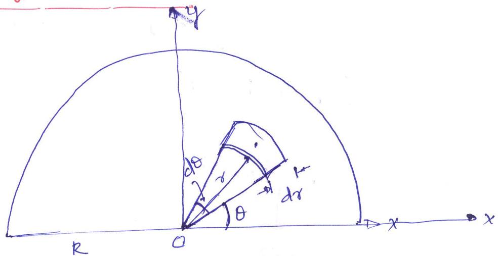
Consider the semicircle of radius  $R$  as shown in figure. Due to symmetry centroid lies on  $y$ -axis. Let its distance from diametral axis be  $\bar{y}$ . To find  $\bar{y}$  consider an element at a distance  $r$  from the centre  $O$  of the semicircle, radial width being  $dr$  and bound by radii at  $\theta$  and  $\theta + d\theta$ .
