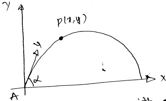
Consider a projectile thrown with a initial velocity  $u$  at angle of  $\alpha$  with respect to horizontal. Let  $P(x, y)$  be the position at any instant of time  $t$ .
