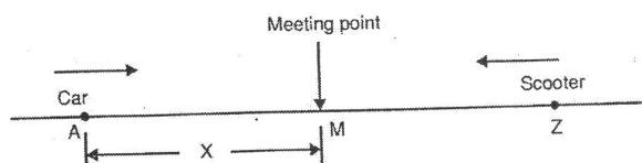
Refer figure. At  $t = 0$ , let the car be at position A and the scooter be at position Z. Let the two vehicles pass each other at M which is  $x$  metres from A,  $t$  sec later.
