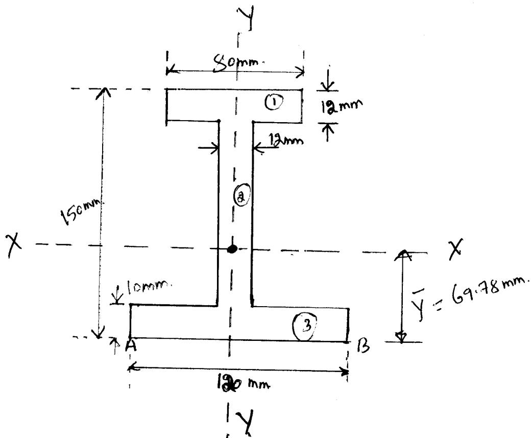
Since section is symmetric about  $y-y$  axis  $\bar{x} = 0$
