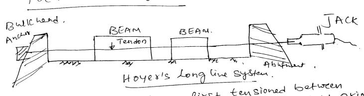
Here The Tendon's one first tensioned between Rigid anchor Blocks, Carst on the ground, prior to the Consting of concrete in the round. When the falling Concrete attains Sufficient Strength, the jalling Drawn. Pressive in released. The tendon's tend to Shorten but are checued by the bond between Concrete & Steel. In this way pre- Stress is to conserve by bond shootenly to ansferred to the Concrete by bond contenty. The bass of prestress is due to claric shootenly of concrete, shortweek & coeff.
