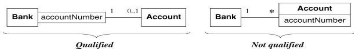
Figure 3.22 Qualified association. Qualification increases the precision of a model.
