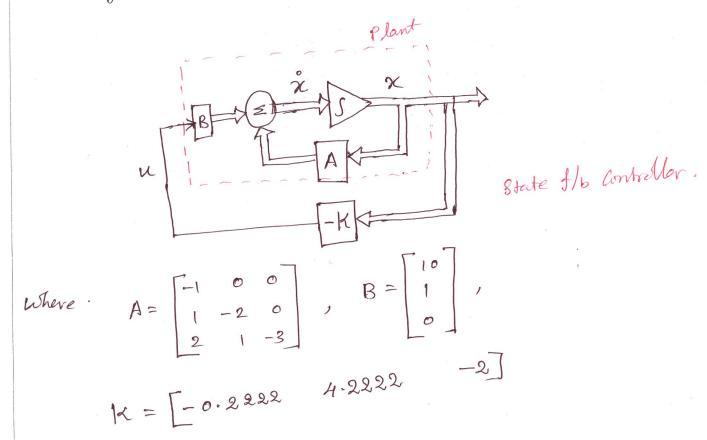
3. Design a full 8tate observer for the following 8ystem at eigen Values  $-2\pm j2\sqrt{3}$  and -5. Draw a block diagram of the 8ystem with 8tate observer.
