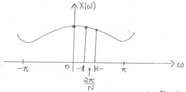
Fig: Frequency sampling of DTFT spectrum at  $\omega = \frac{2\pi k}{N}$ , where  $k=0, 1, \dots, N-1$
