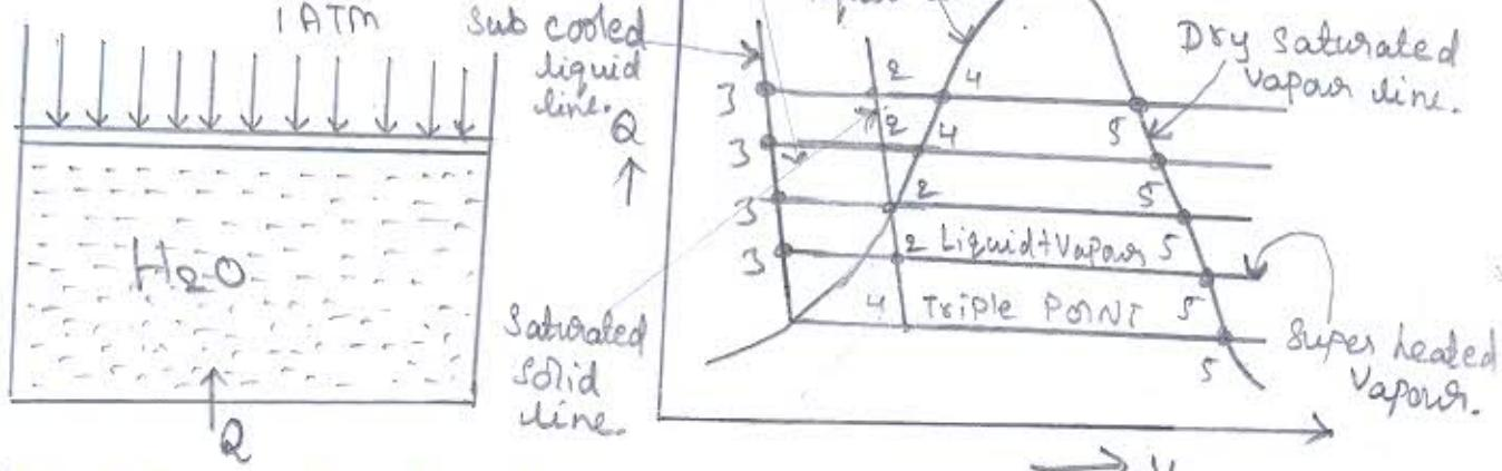
Consider Ice at  $-10^\circ\text{C}$  & 1 atm pressure contained in a cylinder & piston arrangement. Let the ice is heated slowly & change in volume are noted. The following observations are noted during heating of Ice.
