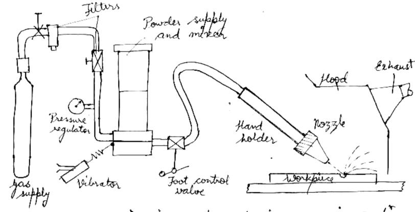
In AJM, air is compressed in an air compo.
