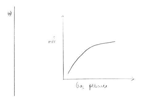
Pariables which offed the 6. Effect of process parameters: MPR, surprise and accuracy of mechined -The MRR or cutting rate increases with increase in both amplitude and vibration of the tool. The amplitude and freg. of vibration determines The velocity of the alrasive particles at the interface by tool and w/p. At amplitudes => K.E. ] => 1 mech-shipping => 1 MRR 1 surface roughness (minimal effect) MRR - Amplitude
