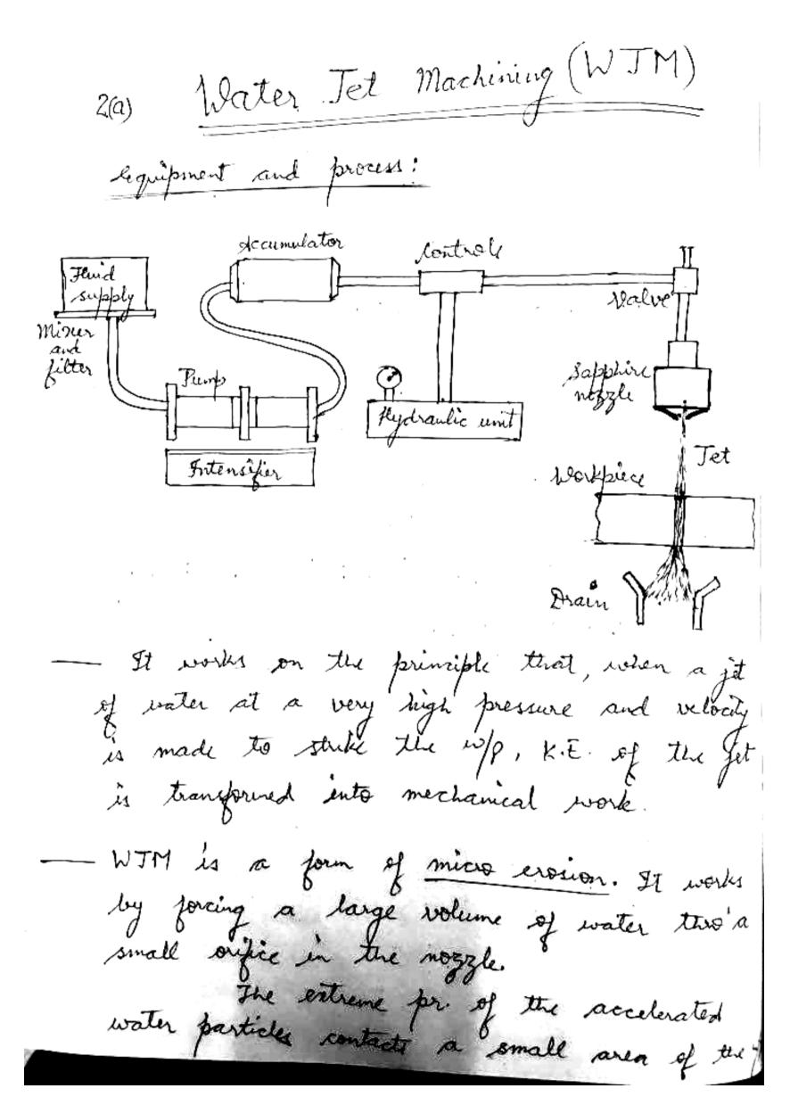
and acts like a saw and cuts a narrow groove in the material.
